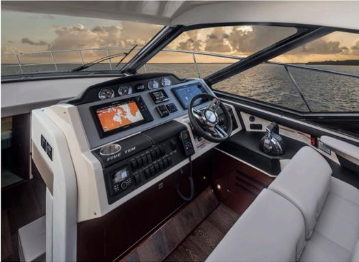
The well-designed control station features standard SmartCraft® diagnostics, VesselView display, plus a Raymarine® Radar/Chartplotter & VHF radio.
