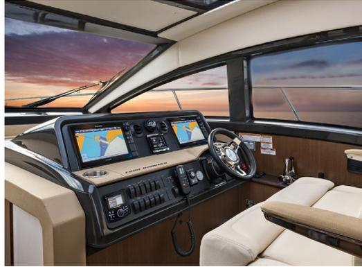
The fully equipped control station features SmartCraft™ diagnostics and VesselView display, plus a Raymarine® eS12 widescreen radar/GPS/chartplotter or optional dual displays.
