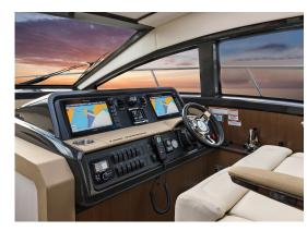
The fully equipped lower control station features SmartCraft™ diagnostics and VesselView display, plus a Raymarine® eS12 widescreen radar/GPS/chartplotter or optional dual displays.
