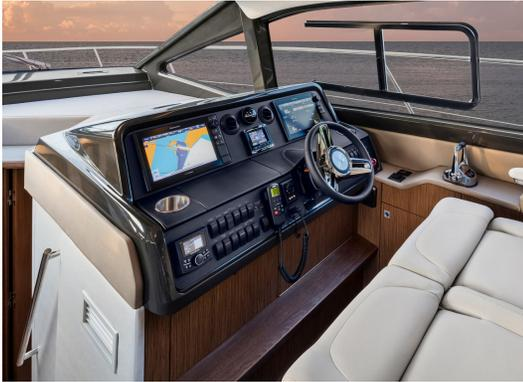
Tiered, instrument panels provide loads of space for the SmartCraft® VesselView display, as well as illuminated rockers and Raymarine® eS12 Radar/Chartplotter combo display.
