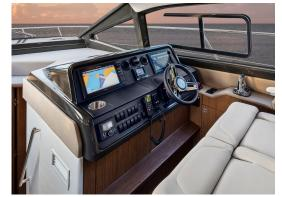
Tiered, instrument panels provide loads of space for the SmartCraft® VesselView display, as well as illuminated rockers and Raymarine® eS12 Radar/ Chartplotter combo display.
